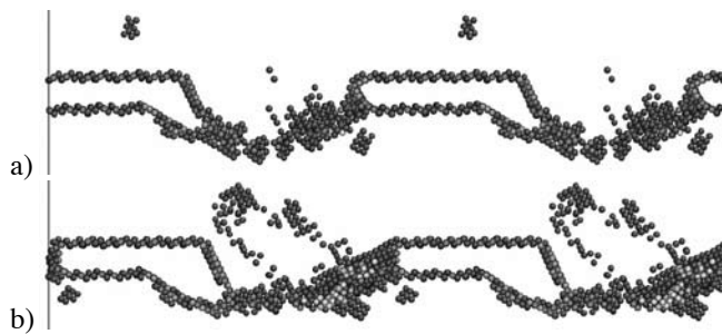
Fig. 9. Detail of the cracked copper bicrystal ( 2a/X = 1/2 ) presenting a symmetrical tilt boundary \Sigma 17(530)/[001] at 300 K with (a) \gamma = 0.11 (before GB slip), and (b) \gamma = 0.138 (after GB slip).
